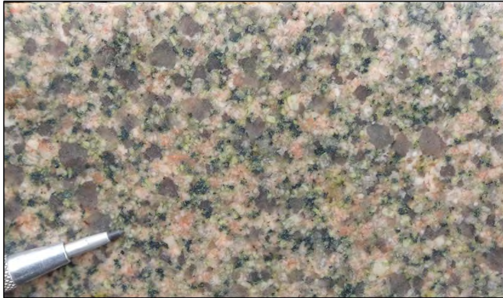
Figure 7.5 Distal Epidote-Chlorite-Weak Hematite Alteration on Granodiorite (from Footwall Zone at Souwa - DPDD1382 @ 103.4 m Depth)
