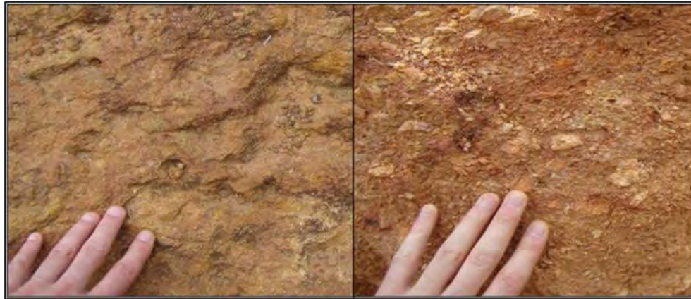
Figure 7.9 Two Examples of Doropo Saprolite Showing Quartz Vein Fragments in the Right Hand Photo
