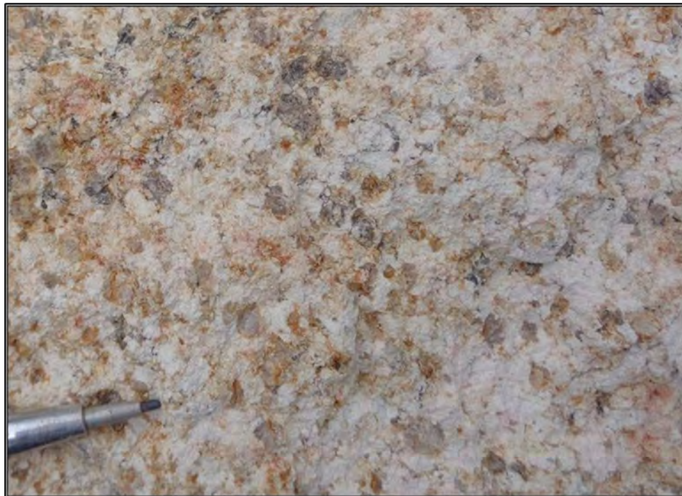
Figure 7.10 Saprock (Original Fabric and Mineralogy is Partially Preserved)
