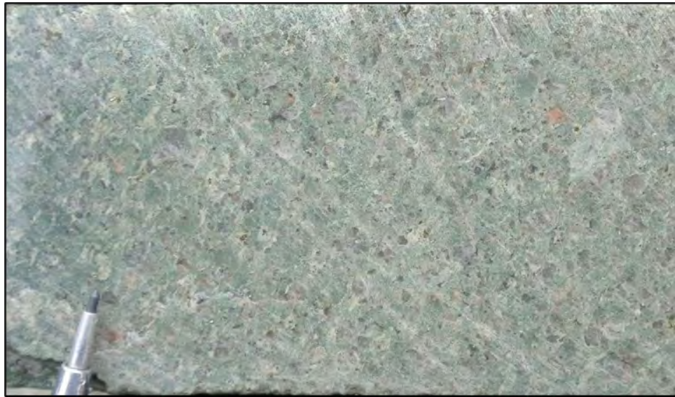
Figure 7.7 Proximal Intense Sericite and Fine Grained Disseminated Pyrite Alteration (from the Han Deposit - DPRD0470 @ 94 m Depth)
