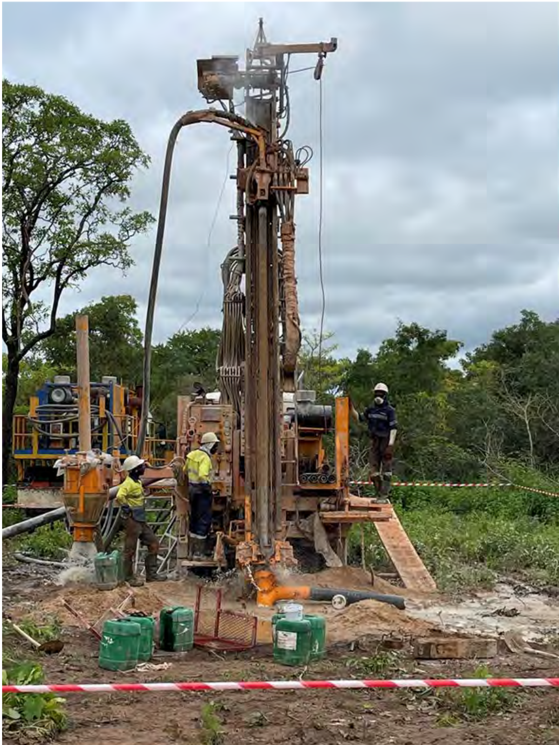
Figure 10.1 The Geodrill UDR650 Multipurpose Drill Rig with Compressor Visible in the Background
