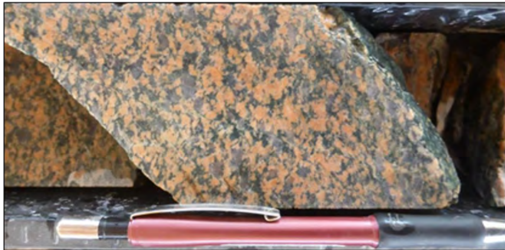
Figure 7.5 Distal Epidote-Chlorite-Weak Hematite Alteration on Granodiorite (from Footwall Zone at Souwa - DPDD1382 @ 103.4 m Depth)
