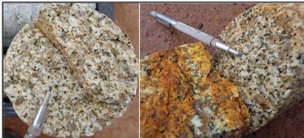
Figure 7.12 Transition Zone Between Lower Saprolite and Fresh Rock
