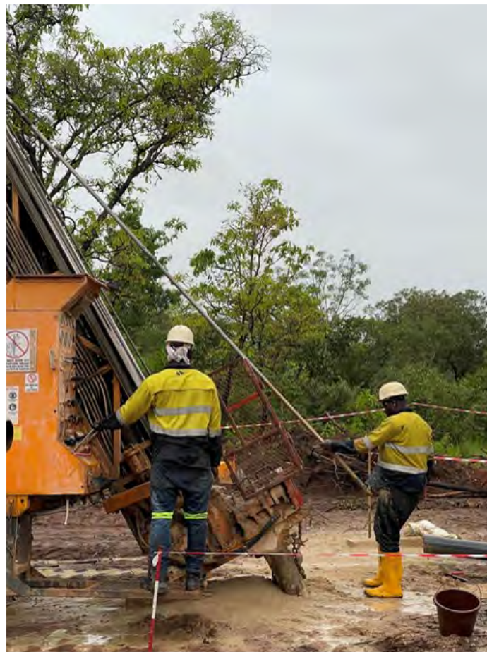
Figure 10.3 The Reflex EZ Shot Tool About to be Inserted into a Drill Hole to Take a Downhole Survey Reading
