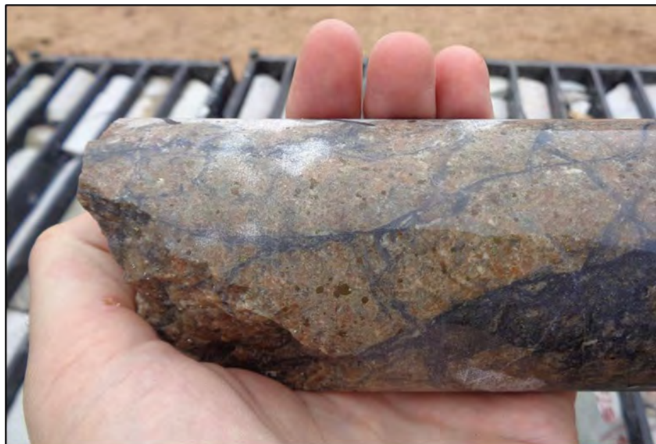
Figure 7.8 Strong Silica-Sericite Alteration - High Grade Mineralisation (from the Han Deposit - DPRD0470 @ 98.7 m Depth)
